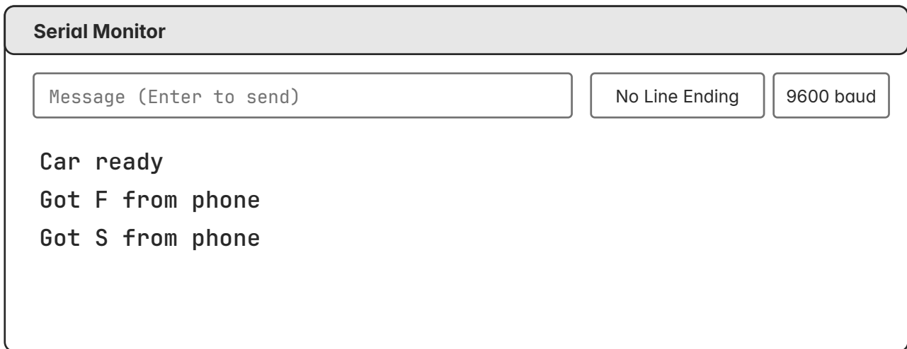
FIGURE 11.2 The Serial Monitor during the round trip. Each letter from the phone is shown as it arrives: Got F from phone, then Got S from phone.
