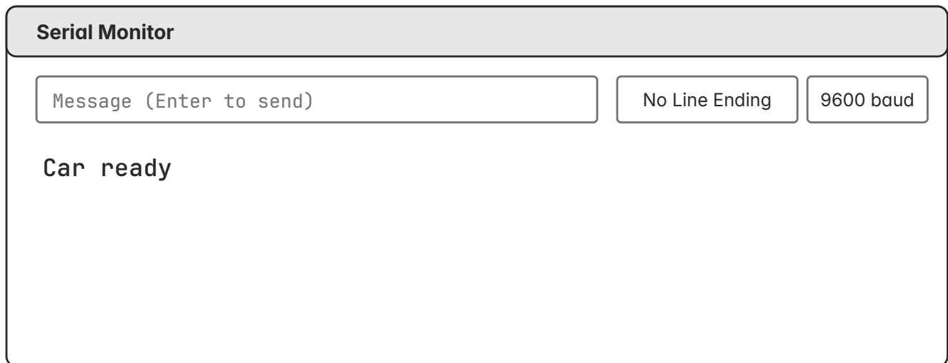
FIGURE 6.1 The Serial Monitor after the upload. It shows the words Car ready, and its speed is set to 9600 baud.
